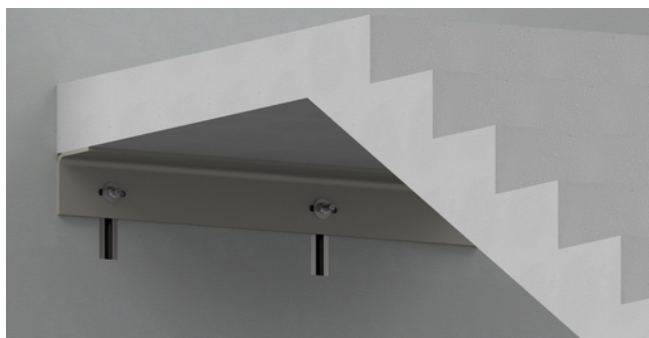
Precast stair support connection
