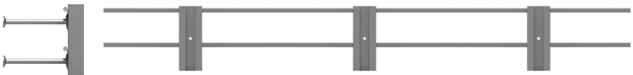
Section and elevation views of a typical Anchor Channel Ladder JXA – LR assembly
