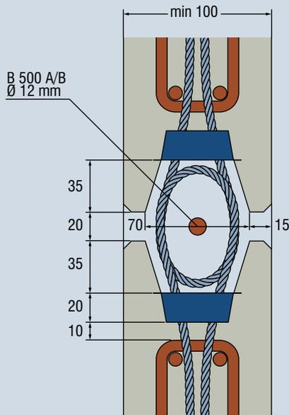
Figure 14: Joint geometry – flat
