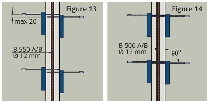
Vertically, the loops are usually to be fitted without any offset, so that they touch one another and lie directly on top of one another (Figure 13). A maximum vertical position tolerance of 20 mm is permitted (Figure 14).
