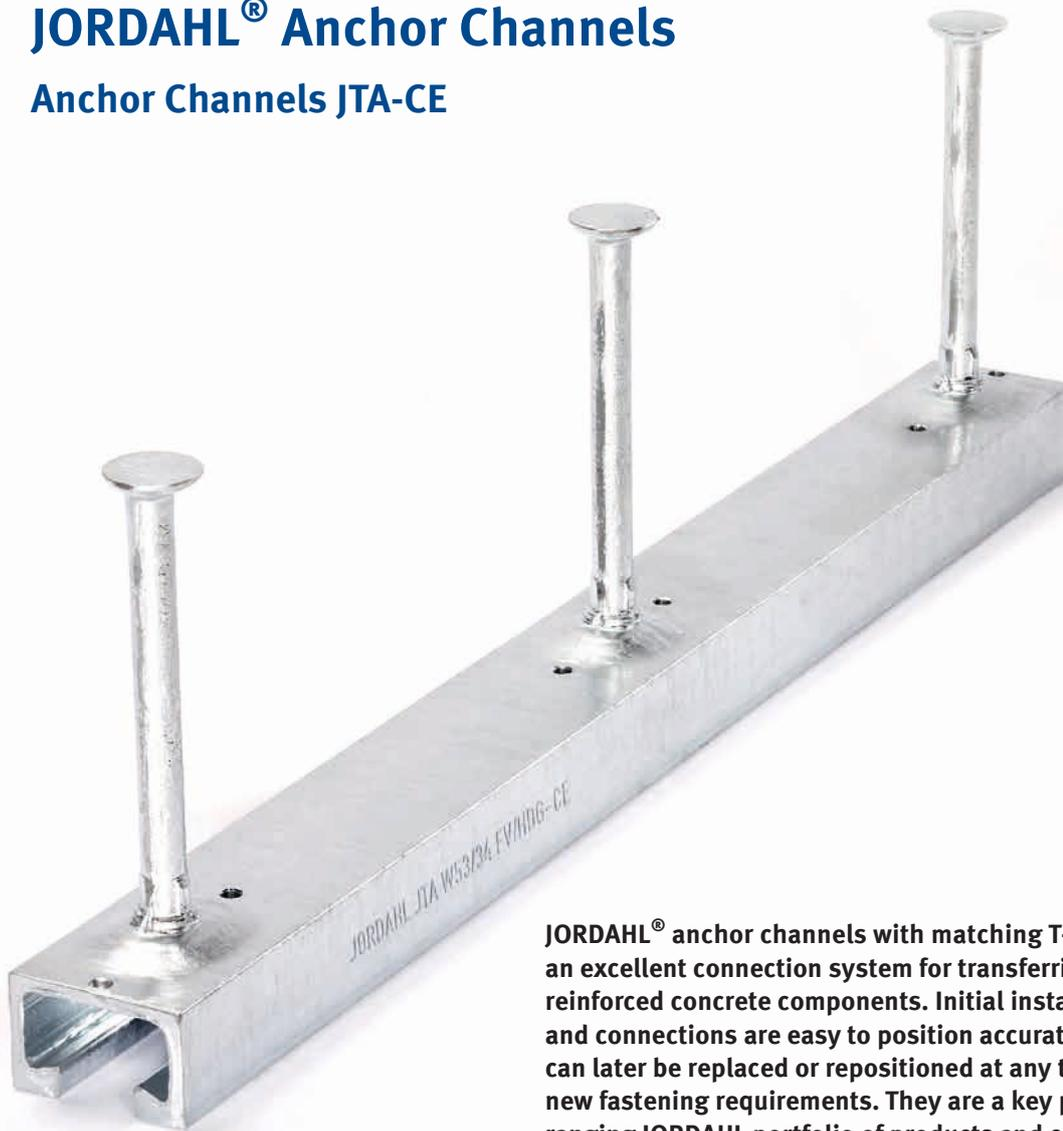
**JORDAHL® anchor channels with matching T-bolts create an excellent connection system for transferring loads to reinforced concrete components. Initial installation is fast and connections are easy to position accurately. Connections can later be replaced or repositioned at any time to match new fastening requirements. They are a key part of the wide-ranging JORDAHL portfolio of products and can be used for a wide variety of different applications.**
