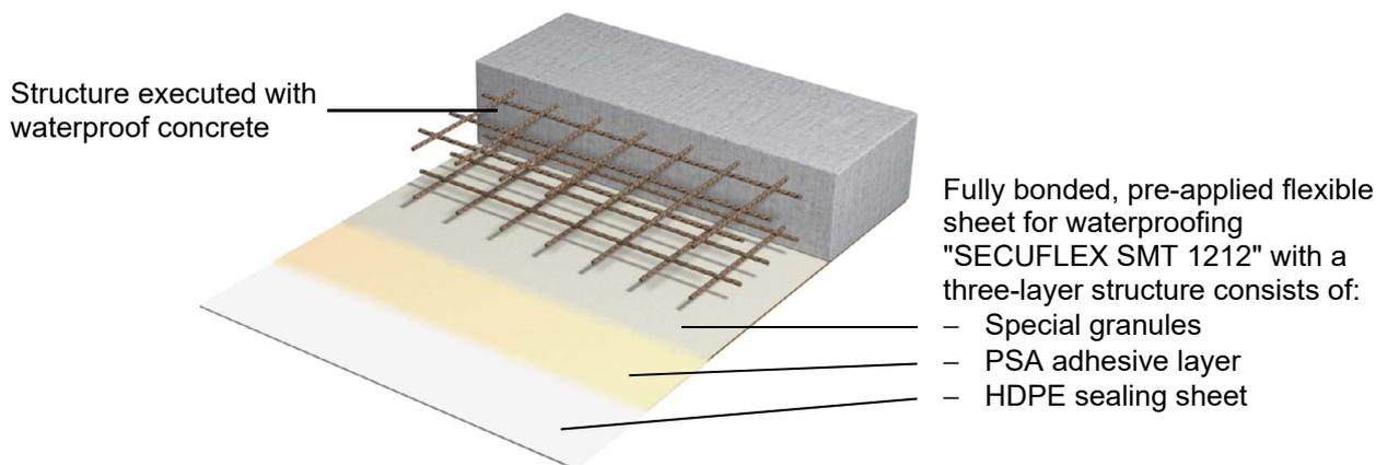
**Additional description of the fully bonded, pre-applied flexible sheet for waterproofing "SECUFLEX SMT 1212"**
